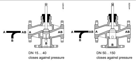
Guided plug which is integrated in the valve stem. The seats are machined in the valve body. Schematic representation, design variations are possible.
