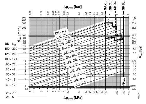
Δp<sub>max</sub> = Maximum permissible differential pressure across the valve (mixing: port A-AB, B-AB, diverting: port AB-A, AB-B), valid for the entire actuating range of the motorized valve
