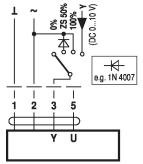
Control remotely 0...100% with positioner SG..
