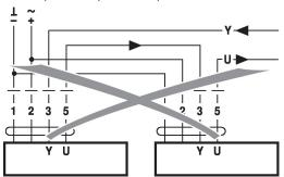
Control with 4...20 mA via external resistor
